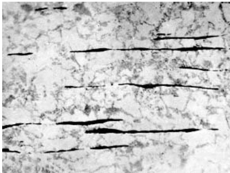
LAMELLAR TEARING SURFACES AT THE EXPOSED PLATE EDGE. (B) REDESIGNED
