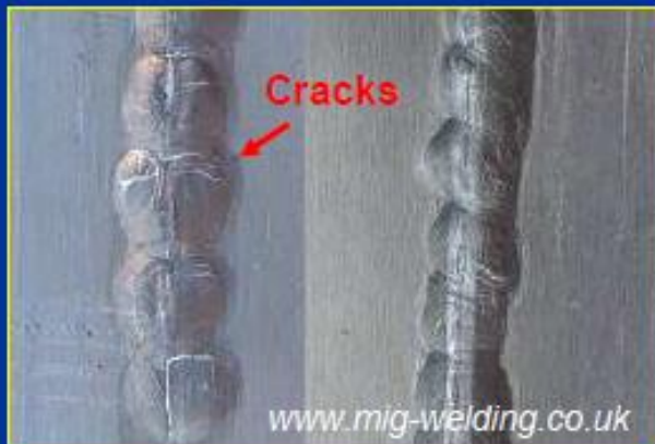
Cracks in aluminium welds
